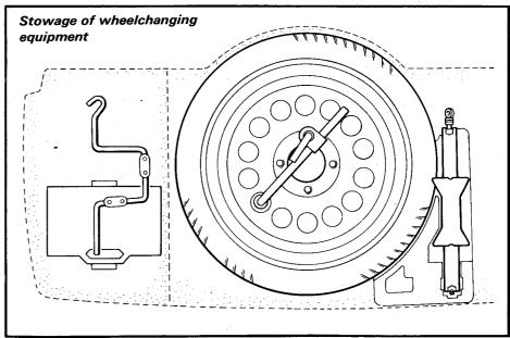
2. The spare wheel, wheelbrace and jack are mounted beneath the boot floor. Pull up the boot floor, and turn the wheel clamping screw counterclockwise to release the spare wheel and wheelbrace. Unclip the jack handle from the underside of the floor, and remove the jack from its location to the right of the spare wheel well.
