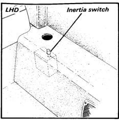
right hand side of the roof stowage compartment floor, and on left hand drive cars, beneath the left hand speaker trim panel. The switch may be reset by pressing down the plunger which pops up when the switch is triggered, with an access grommet provided for this purpose on left hand drive cars.
