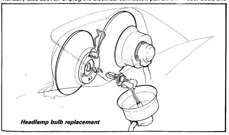
unhook the wire spring clip securing the halogen bulb. **NOTE** – Do not touch any part of a halogen bulb glass envelope with the fingers, as the greasy deposit left behind will drastically shorten the bulb's life.
