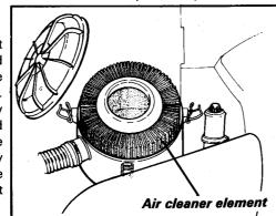
Before removing the filter element, the precaution should be taken of disconnecting the engine intake hose from the filter box in order to prevent any possibility of dirt entering the hose and engine. The filter element may then be withdrawn from the housing after releasing the four over-centre clips, and removing the lid. Thoroughly clean out the inside of the filter box before fitting a new element, ensuring that it is correctly seated. Refit the cover lid, and engine intake hose.
