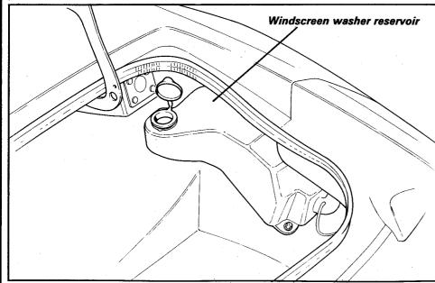
If the washer fluid level becomes low, and needs replenishing, an amber tell tale reminder in the instrument panel will glow.
